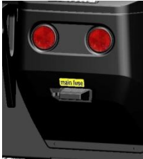
position of the main fuse
