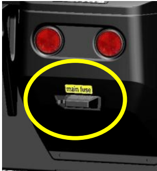
place of the main fuse
