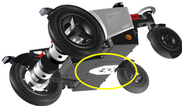
EvO chassis with Dahl Docking plate mounted.
