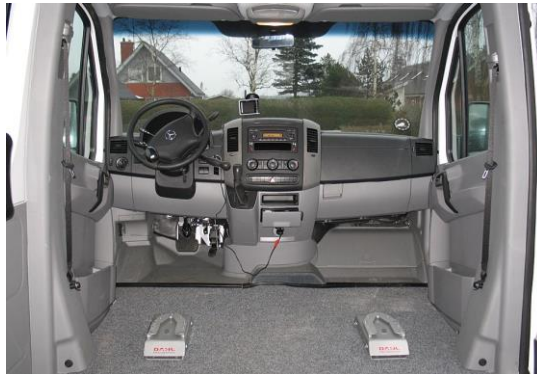
Dahl docking station mounted on the floor
