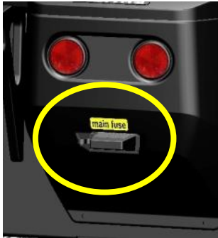
place of the main fuse
