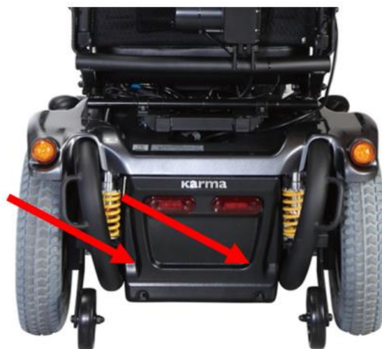
position of the battery pole (behind the rear cover)
