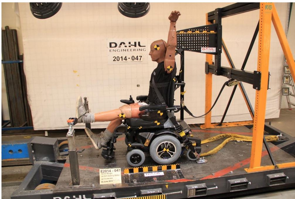
Morgan crash test using Dahl Docking station.
