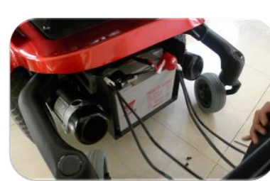
position of the rear battery (behind both covers)
