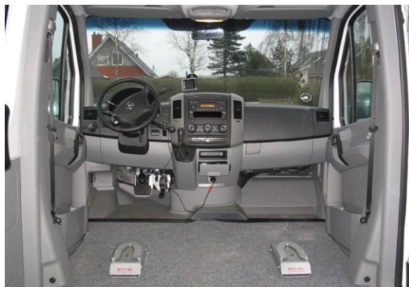
Dahl docking station mounted on the floor
