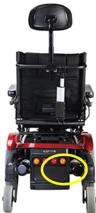
position of the serial number sticker
