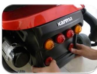
position of the rear battery (behind both covers)
