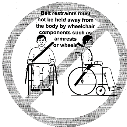
Figure 6 — Illustration of improper belt-restraint fit
