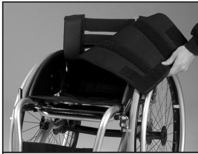
Image 22 Fold the back of the upholstery
