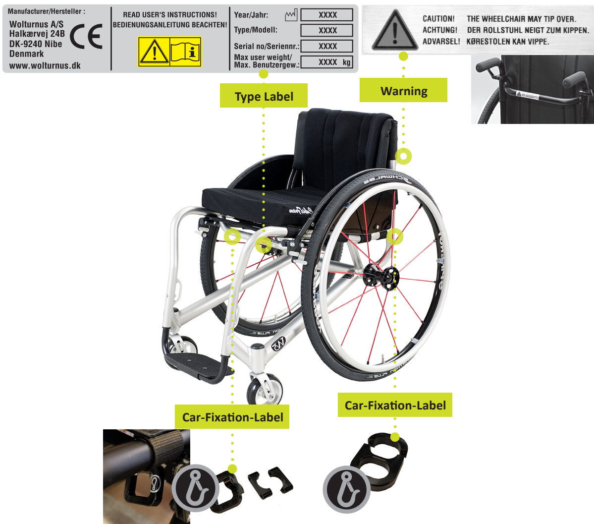
Image 1 Location of type labels, anti-tip warnings, and restraining points
