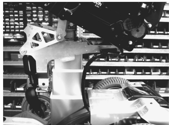
Fig. 6-77 Lifter column completely extended
