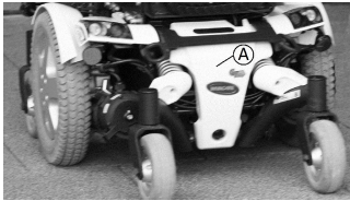
Power module behind rear shroud (A) Fig. 6-2
