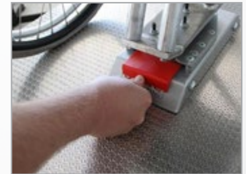
Fig. 50: Manual release step 2
