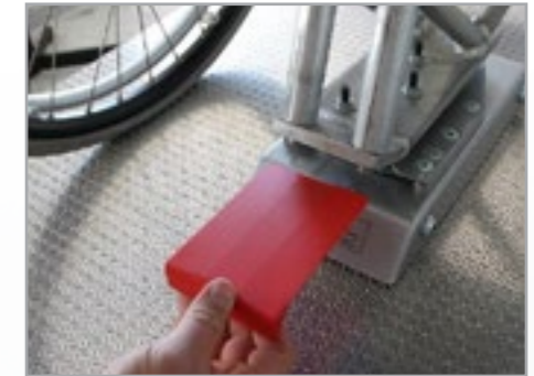
Fig. 49: Manual release step 1
