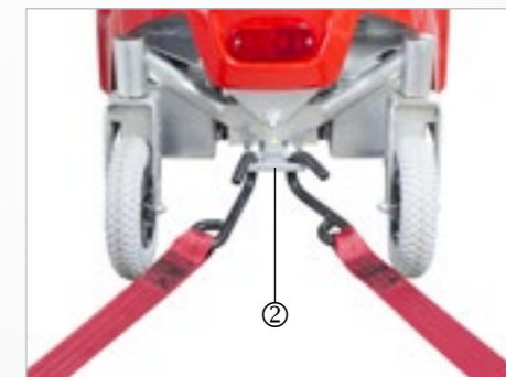
Fig. 29: Securing point at rear
