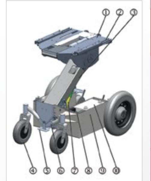
Fig. 11: Components, rear of chassis
