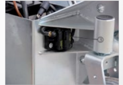
Fig. 111: Main safety switch
