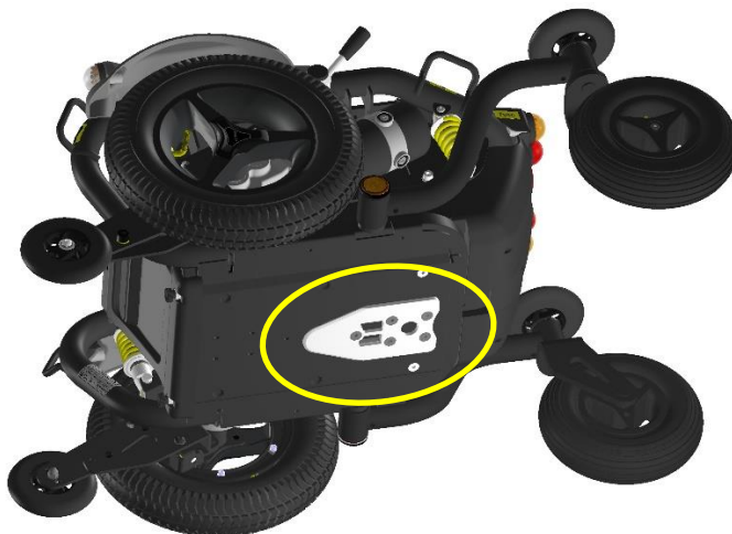
Leon FWD chassis with Dahl Docking plate mounted.
