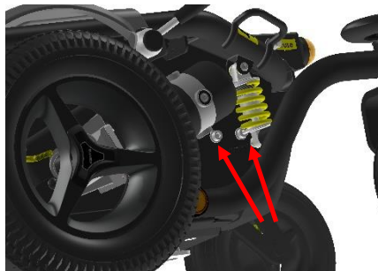
removing the locking bolts
