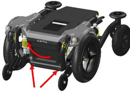
removing the cover bolts
