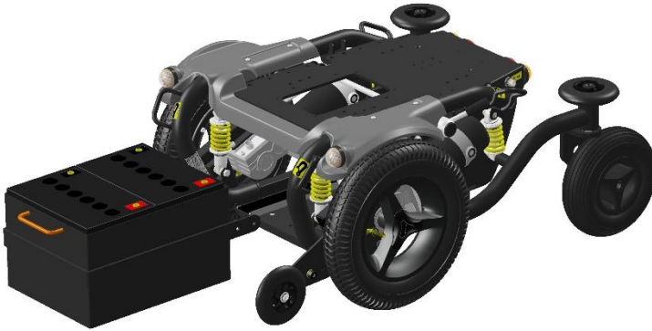
Battery box slides out of the chassis
