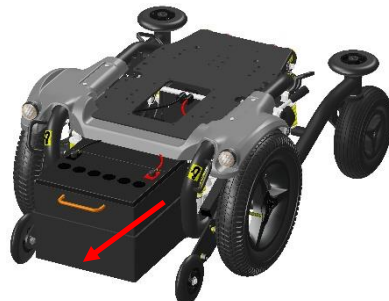
pulling out the battery box
