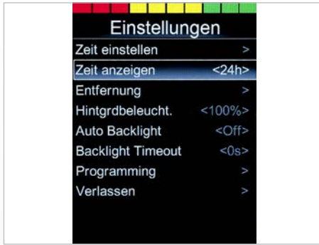
Fig. 73: Set clock to visible/invisible
