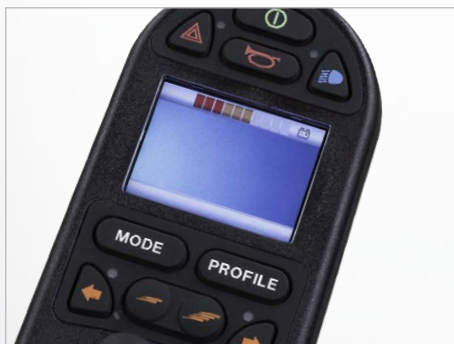
Fig. 89: Driving function blocked
