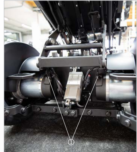
Fig. 27: Brake lock release lever (emergency release)
