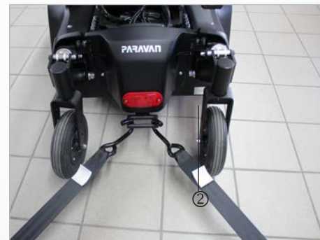
Fig. 33: Attachment point at the rear
