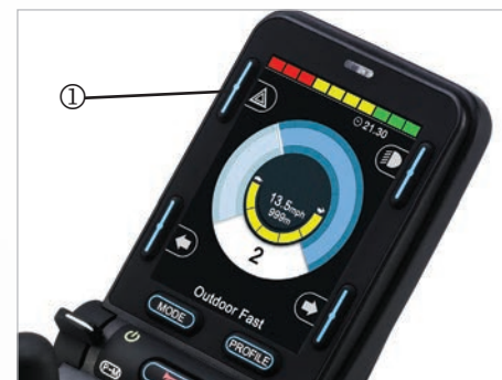
Fig. 62: Hazard lights on / off
