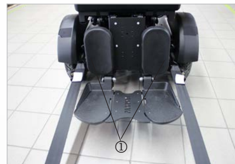
Fig. 32: Attachment point at the front
