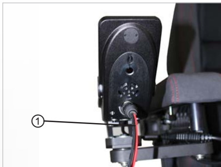
Fig. 109: Plug in the charging cable
