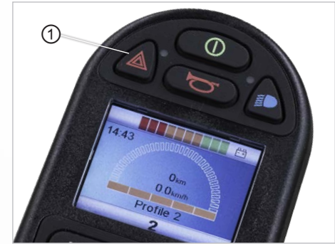
Fig. 86: Hazard lights on / off
