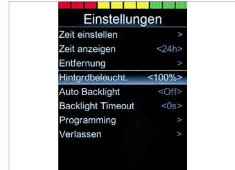
Fig. 74: Setting the display brightness
