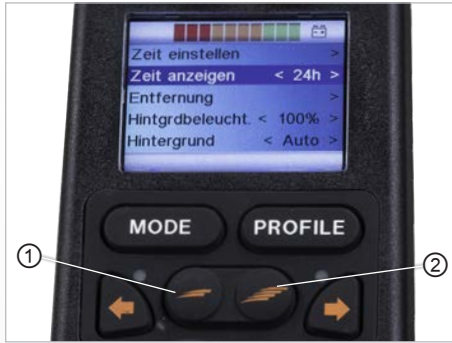
Fig. 97: Set clock to visible/invisible
