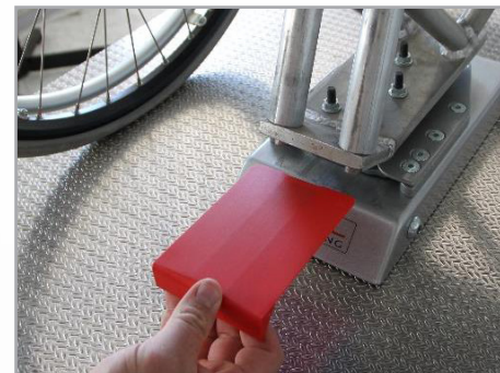
Fig. 52: Manual unlocking step 1
