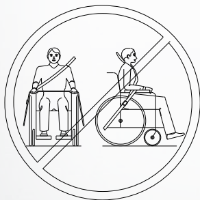
Fig. 34: Illustration of an inadequate belt system
