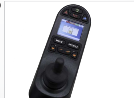
Fig. 101: Controls blocked – block symbol
