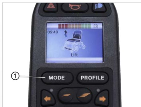
Fig. 92: Display of seat functions
