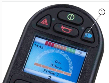
Fig. 74: Light on and off
