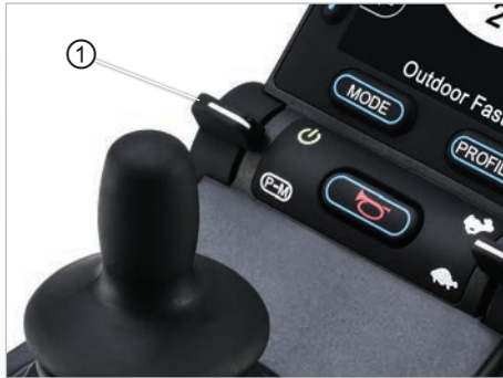
Fig. 50: Speed control (tortoise) active
