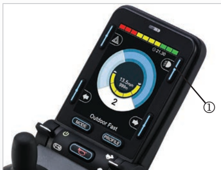
Fig. 52: Light on and off
