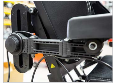
Fig. 13: Angle of armrest pad
