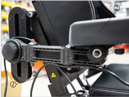
Fig. 14: Position of the armrest pad
