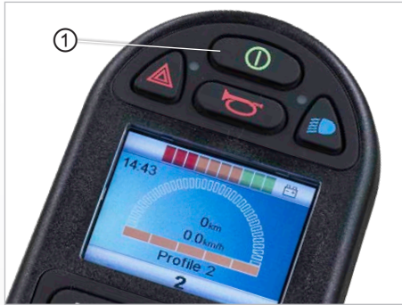
Fig. 72: "On / off" key
