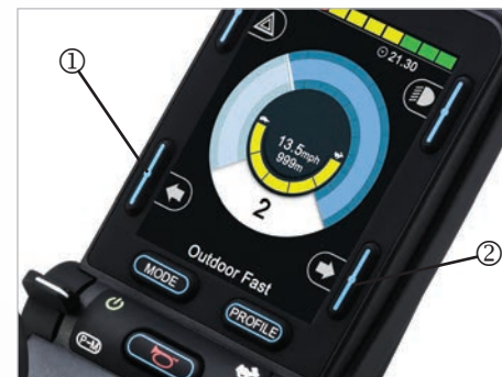
Fig. 53: Turn signal right / left
