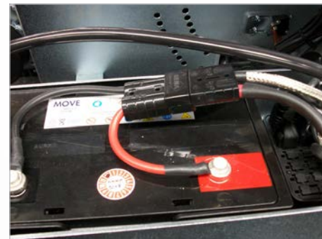
Fig. 40: Main cable battery
