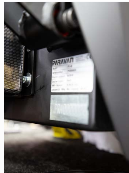
Fig. 6: Location of type plate
