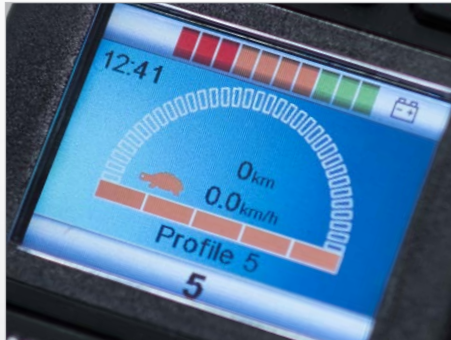
Fig. 73: Speed control (tortoise) active
