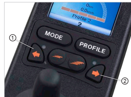
Fig. 75: Turn signal right / left
