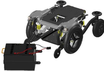
unplugging the cables
