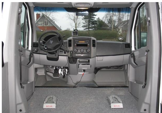
Dahl docking station mounted on the floor
