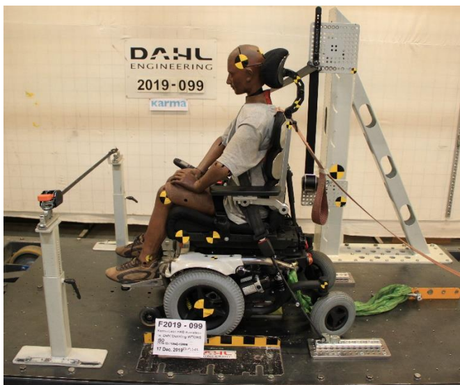
Leon FWD Versus crash test using Dahl Docking station.
