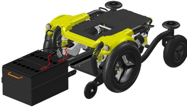
Battery box slides out of the chassis
