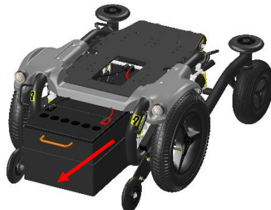
pulling out the battery box
