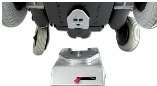
Docking station and docking plate on chassis
