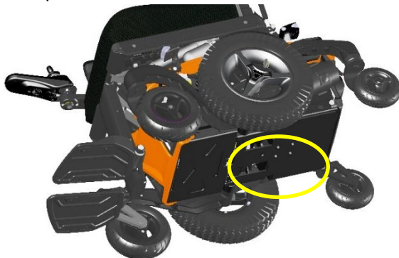
Dedicated holes for mounting Dahl lock plate
