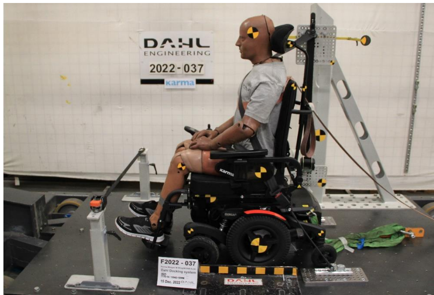
Morgan M Sling (MGNM-SLN) crash test using Dahl docking station
