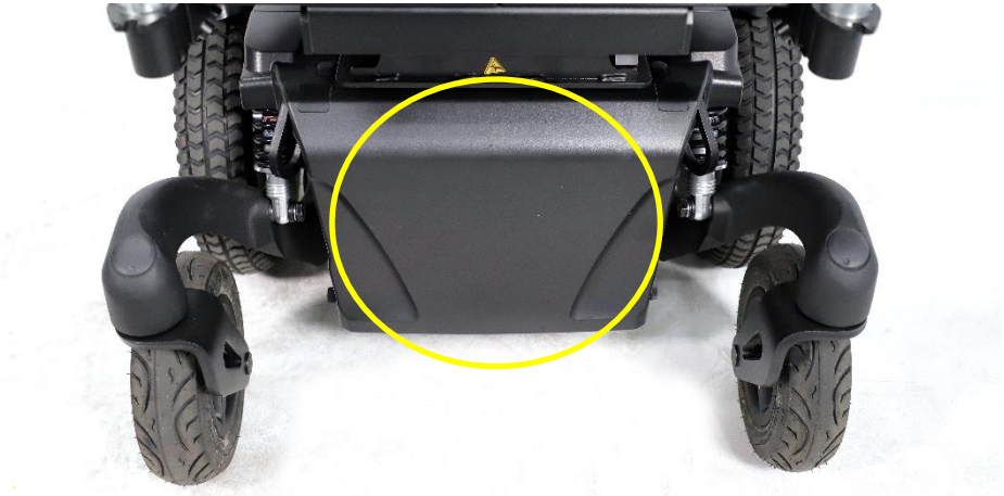
Front battery box
