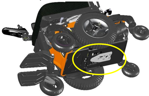
Morgan M Sling (MGNM-SLN) chassis with Dahl lock plate mounted.
