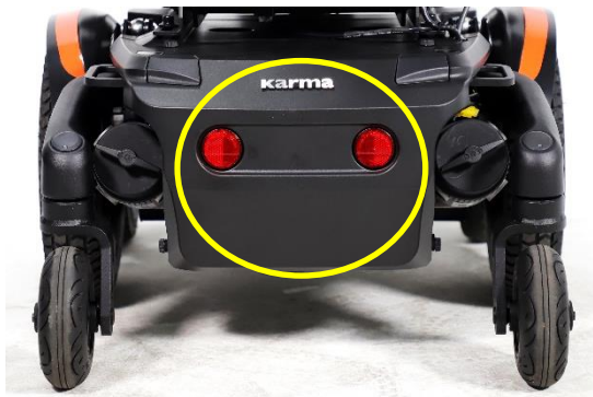
Position of the rear battery box
