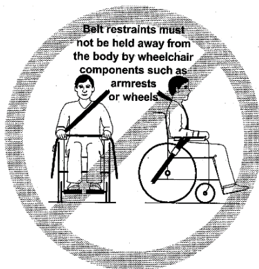
Illustration of improper belt-restraint fit
