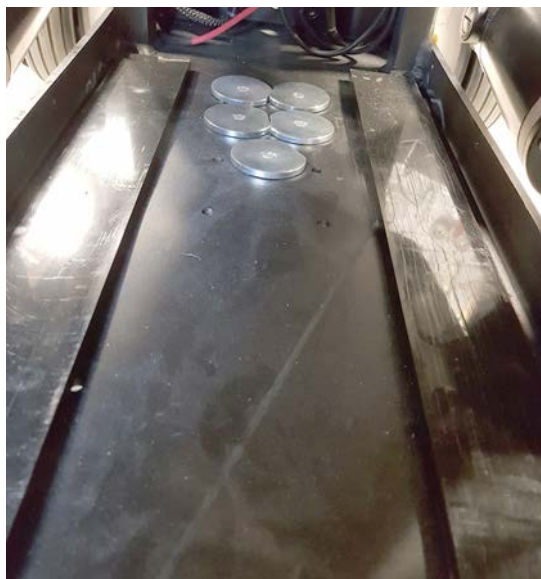
Place the two plates on each side of the nuts. Fix them with double sided tape or a little glue.
