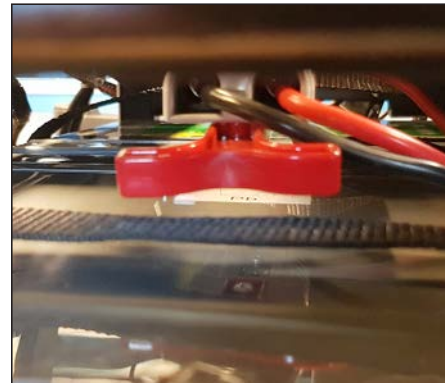
Release the plug by pulling the red handle.
