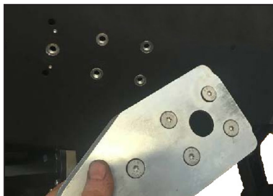
Place the screws included in the set in the locking plate, and mount them in the nuts.
