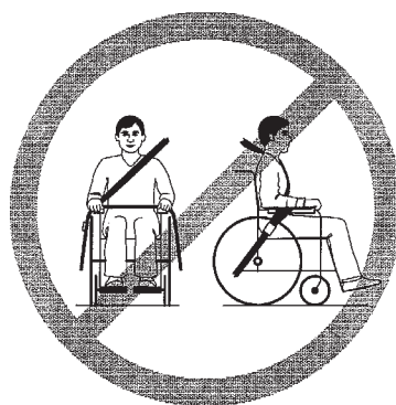
Incorrect use of belts
