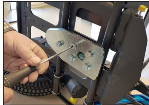
The lock plate should point forward.
