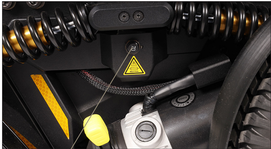
The automatic fuse is placed here.
