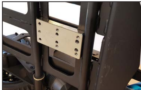
The thick mounting plate is fixed with the screws from the mounting plate on the inside of the battery box. The remaining threaded holes are used when installing the locking plate.
