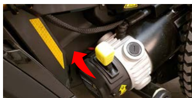
Normal position for driving - pushed up
