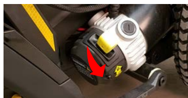
Position for disengagement - pushed down
