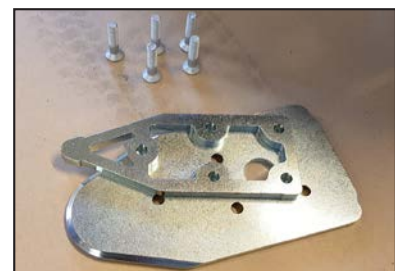
Now we have to mount the 8 mm distance plate and the locking plate with screws from Dahl Docking. Included in Art. no. 501750 and 503600.
