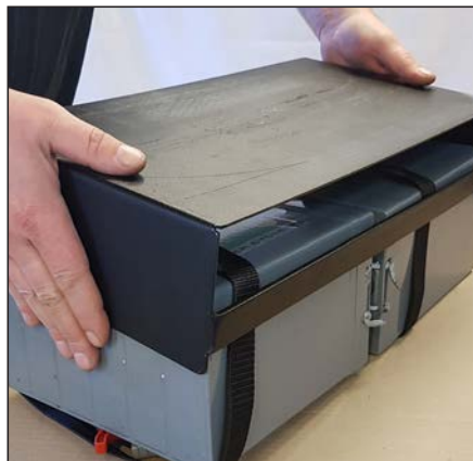
Place the battery box on top, and turn it around.
