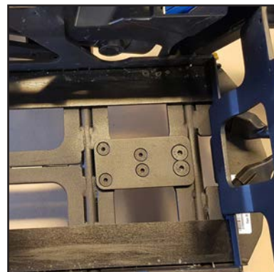
The 2 supplied plates are placed on either side of the mounting plate inside the battery box and fixed with double-sided tape or glue.
