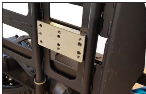
The thick mounting plate is fixed with the screws from the fixing plate on the inside of the battery box. The remaining threaded holes are used when installing the locking plate.
