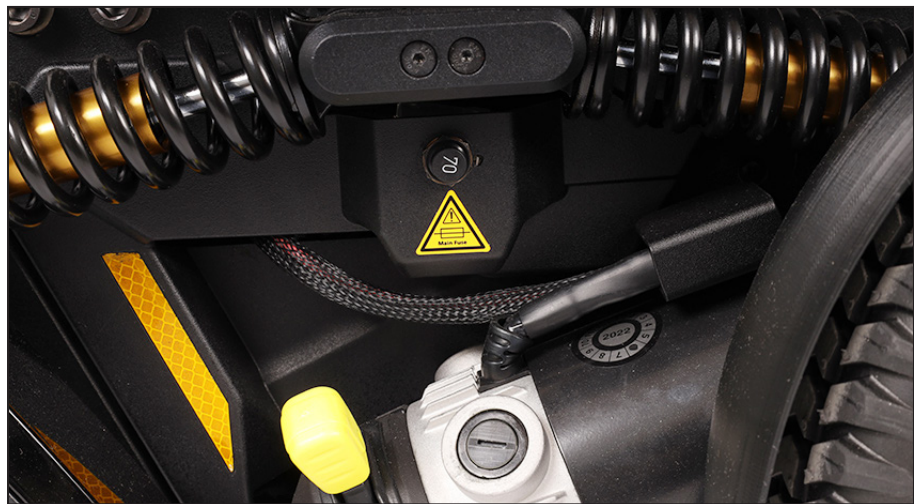
The automatic fuse is placed here.
