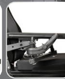
FOLD-UP ARMRESTS and control box that can be swiveled back provide easier access and positioning.
