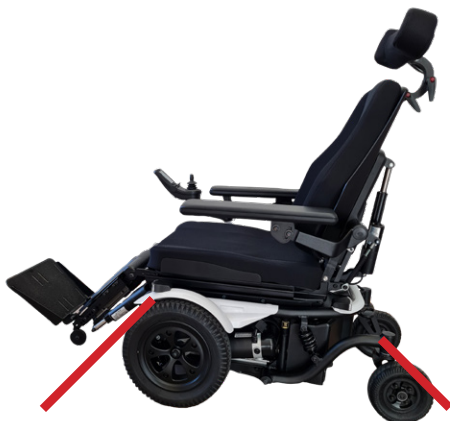
Tie down straps under 45° angle.
