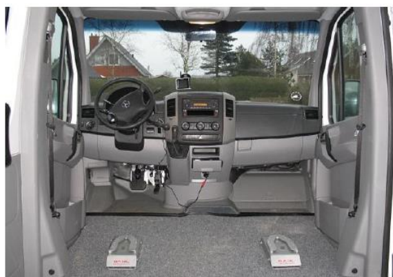
Dahl docking station mounted on the floor
