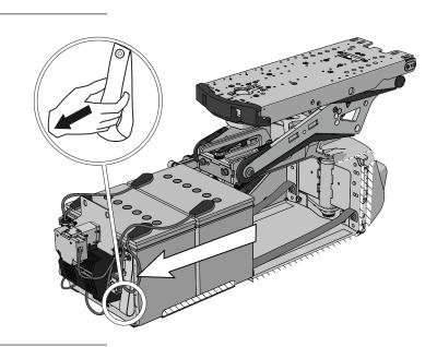
Loosen the two screws that holds the battery box straps inside the chassis. Carefully remove the heavy battery box out of the chassis.
