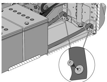
**24** Push the battery box into the chassis.
