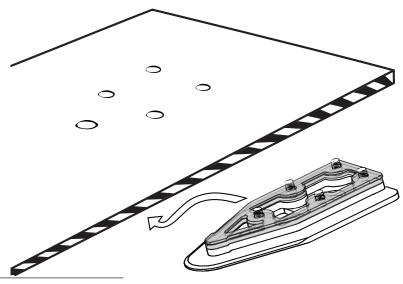
**23** Reattach the two battery box straps with the screws and the washers. Tightening torque: 2.9 Nm/2.14 lb.ft.
