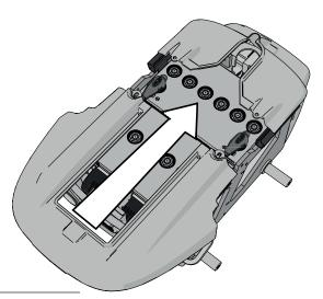
30 Turn the cover knobs without tightening them. Press the top cover and the front chassis cover against each other until any space between them is eliminated. Tighten the knobs by hand.
