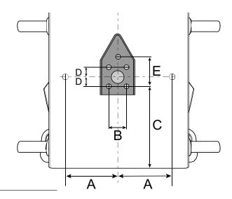
12 Use the lock plate as a template and make marks for the lock plate's five holes in the chassis. Make sure that the lock plate's rear end is parallel with the rear end of the chassis box.
