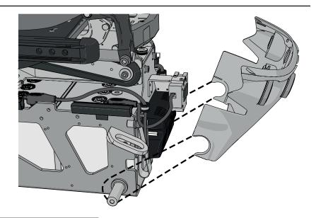
29 Slide the top cover onto the chassis and at the same time push the rear edge of the cover downwards. Make sure it hooks onto the rear cover.
