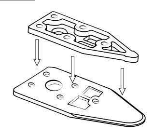
Use more spacers to achieve desired thickness with regards to, for instance, user weight and tire pressure.
