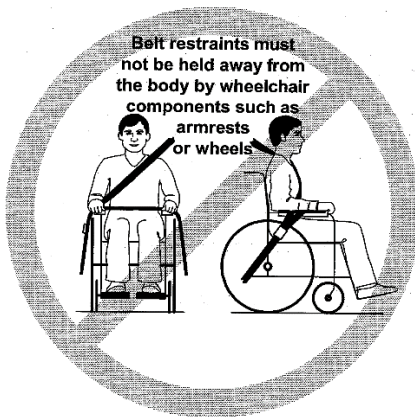
Figure 6 — Illustration of improper belt-restraint fit
