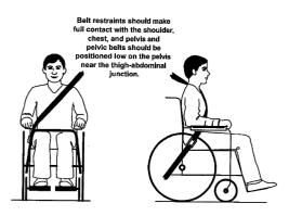
Figure 7 — Illustration of proper belt-restraint fit
