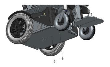
1. Remove the 2 bolts under the lift, see diagram.
