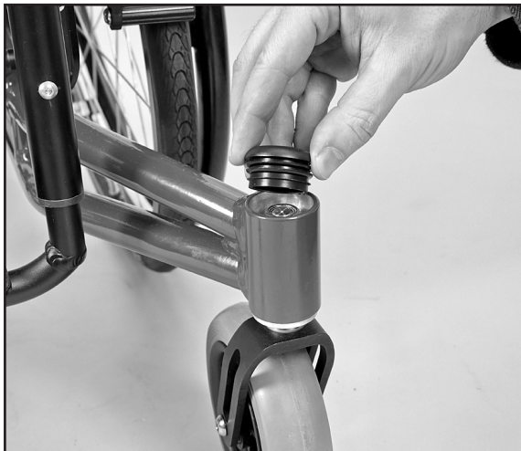
Fig. 51 Remove plastic plug
