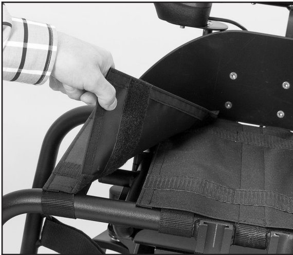
Fig. 18 Loosen the front seat cushion
