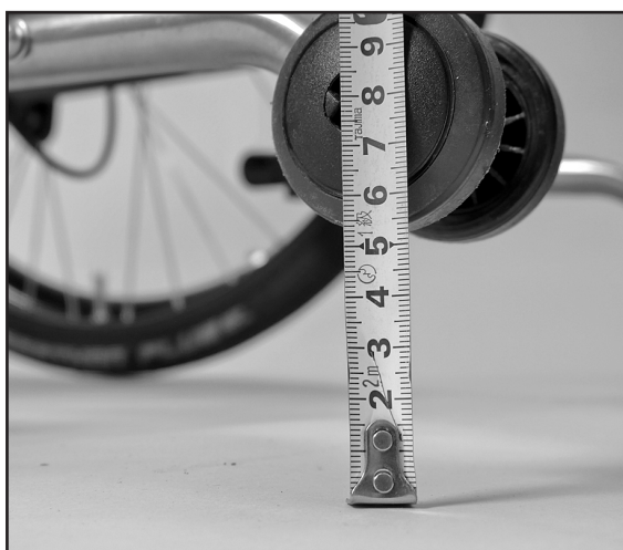
Fig. 36 measuring from floor to anti-tip
