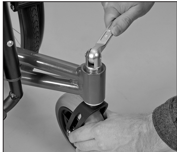
Fig. 52 Unscrew the nut
