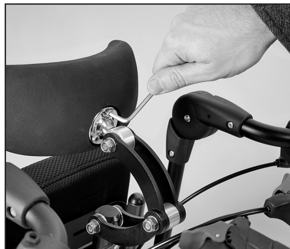
Fig. 11 Adjustment of headrest
