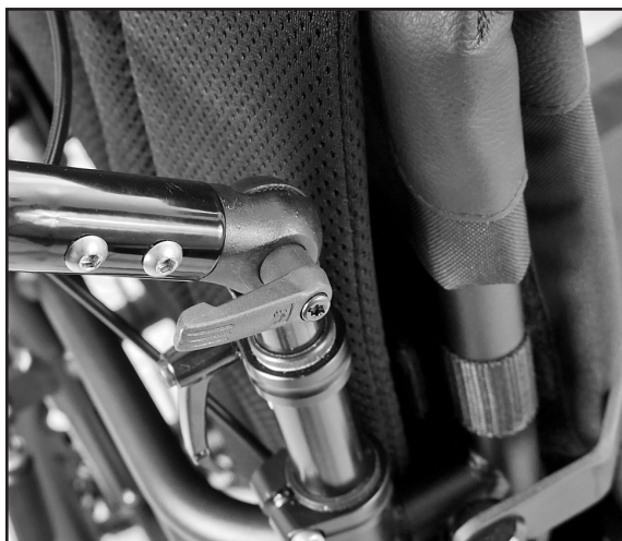
Fig. 14 Loosen handle on both sides
