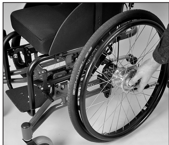
Fig. 31 Mount the rear wheels
