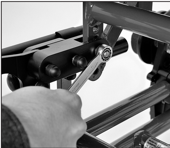
Fig. 16 Remove adjustment bolts
