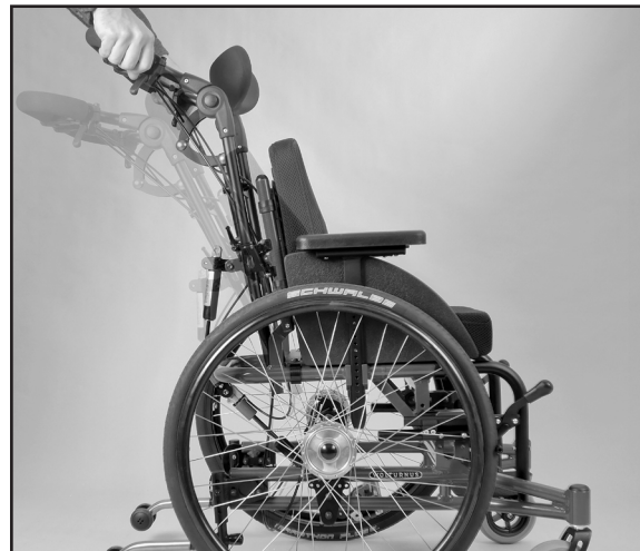
Fig. 46 Adjust back angle
