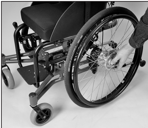
Fig. 28 Remove the rear wheels
