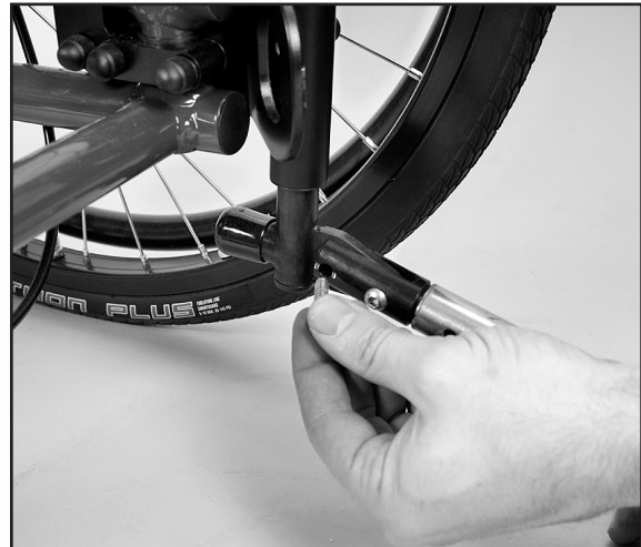
Fig. 40 Adjust guard arm
