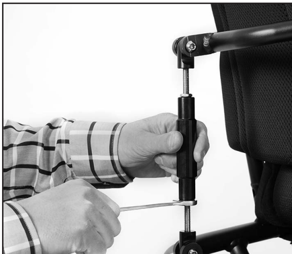
Fig. 7 Loosen nuts on the vane screw
