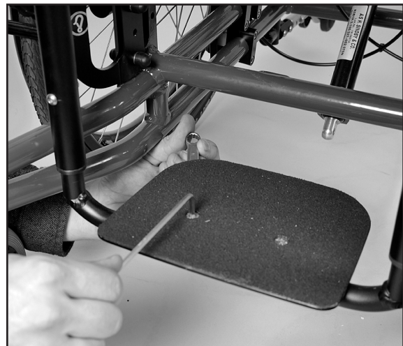
Fig. 34 Loosen the nuts on the footrest
