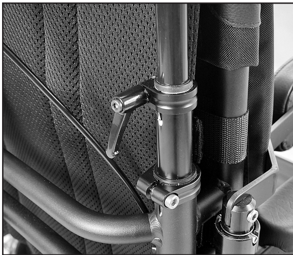
Fig. 12 Loosne handle on both sides
