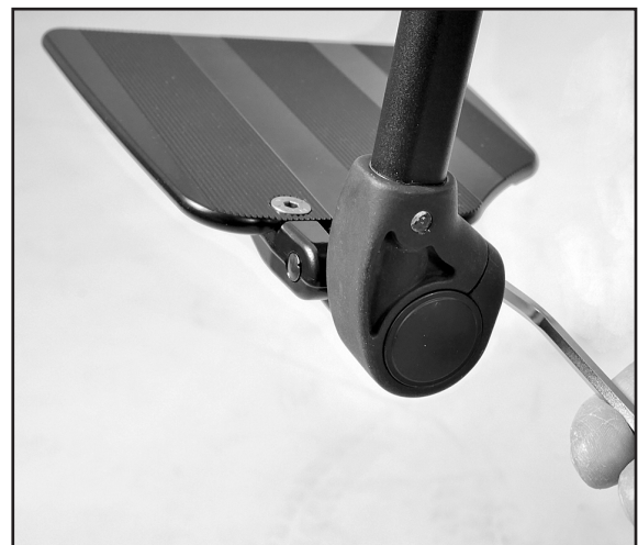
Fig. 35 Loosen the bolts
