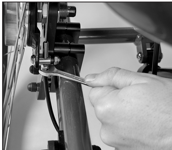
Fig. 44 Adjustment of brakes
