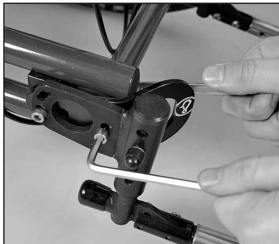
Fig. 41 Remove the three bolts
