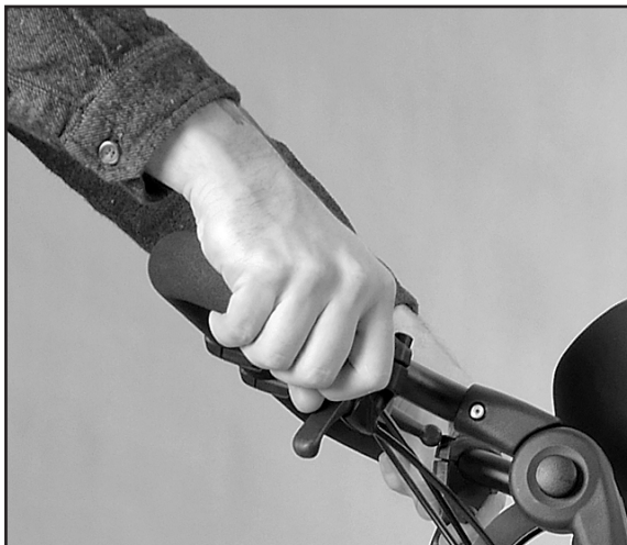
Fig. 24 Hold down the release lever
