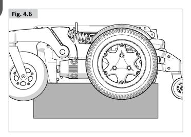
2. Undo the 3 nuts and remove drive wheel (Fig. 4.7).
