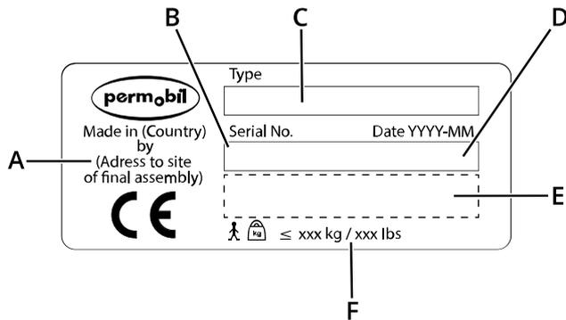
The serial number label is located on the lower, left-hand side of the wheelchair chassis. Look to the right of the drive wheel.
