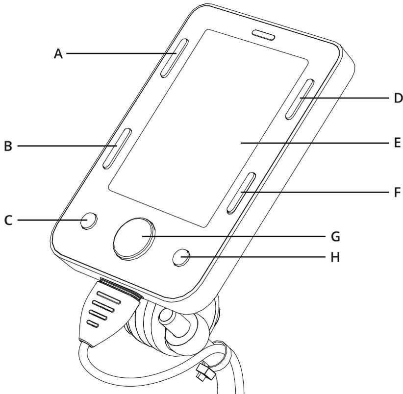
Your wheelchair can be equipped with an Omni2. An Omni2 is a device that makes it possible to operate the wheelchair with something other than a standard joystick.
