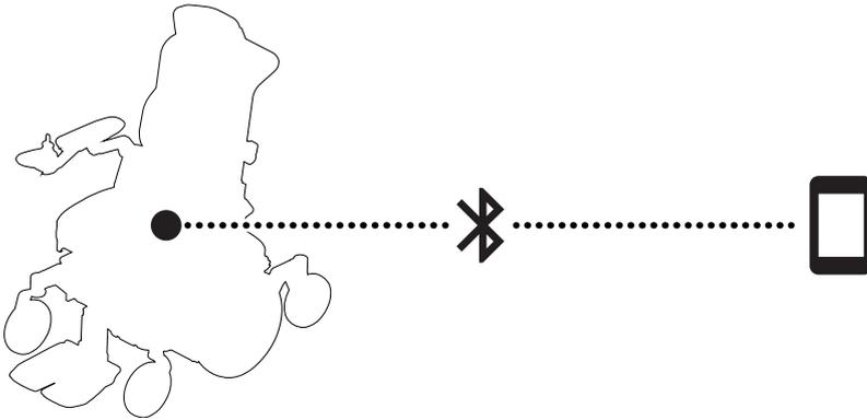
ConnectMe contains a radio transmitter. In certain areas, radio transmission is not allowed and ConnectMe must be set to flight mode ✕.
