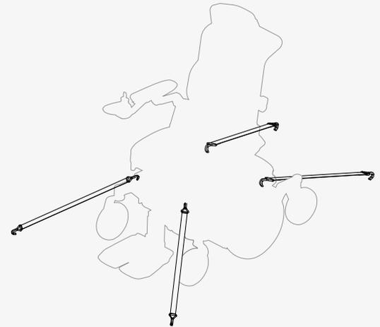
You can also use a docking system to secure your wheelchair. The Dahl docking station is an approved docking system. See the Dahl docking station's manual on how to operate it.
