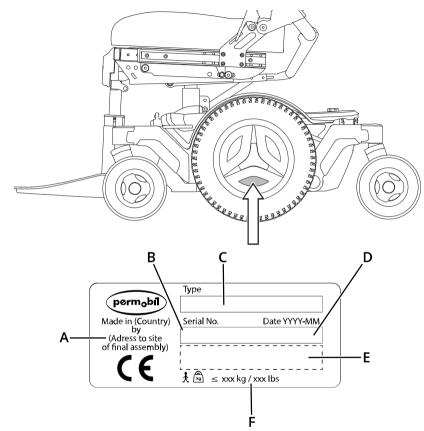
The serial number label is located on the lower, left-hand side of the wheelchair chassis. Look between the rim spokes.
