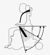
Cover the control panel and other sensitive objects with soft, shock-absorbing material (foam plastic or similar). Push the control panel toward the backrest. Tape any loose cables to the seat or hoods.
