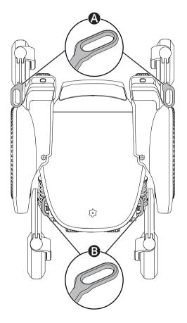
The wheelchair is equipped with four tie-down points used for transportation  $\blacksquare \checkmark \blacksquare$ . Two in the front O and two in the rear O.
