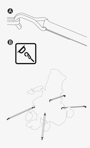
You can also use a docking system to secure your wheelchair. The Dahl docking station is an approved docking system. See the Dahl docking station's manual on how to operate it.
