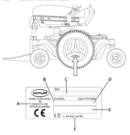
The serial number label is located on the lower, left-hand side of the wheelchair chassis. Look between the rim spokes.
