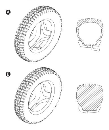
The wheelchair drive wheels have pneumatic tyres or flat-free (foam filled) tyres. The castor wheels have pneumatic tyres or solid polyurethane tyres.
