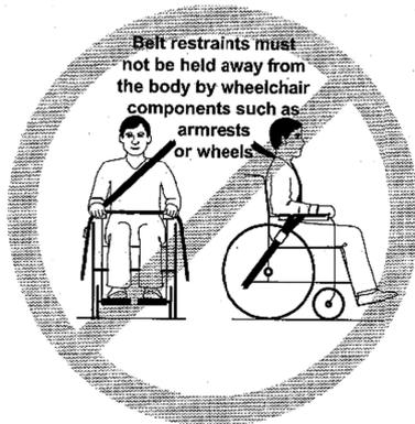
Figure 6 — Illustration of improper belt-restraint fit
