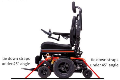
The straps have to be connected to the vehicle at suitable anchor points. Make sure that the tire pressure is at the recommended level so the straps can have maximum effect. Make sure the straps are tightened to maintain optimal security.
