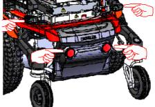
The chassis has very strong and bright LED lights to make sure you can have a safe drive in the dark. The orange reflectors on both sides and the red reflectors on the rear also make you visible for other people as well. The lights fulfill the European requirements. (E marked)
