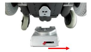
To unlock the docking station manually, the red lever needs to be pulled to the right. This retracts the locking bolt manually so the wheelchair can be released out of the docking station.
