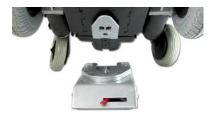
Docking station and docking plate on chassis
