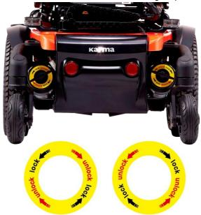
Look for the black lever on each of the driving motor locked at the rear of the chassis.
