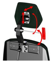
step 2: Loosen up the bolts using a 6mm Allen key. Loosen then up until the headrest can be moved.
