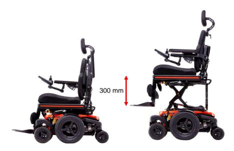
Whilst lifting the seat, the driving speed will automatically reduce to gain maximum stability at all times. At high seating position also the seat tilt will be blocked to gain maximum stability. The seat height can be set to every height position by the user. The maximum seat height is set to 760 mm (seat pan to ground)
