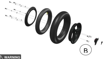
Do not loosen the central hub bolt to remove the front wheel.
