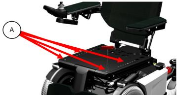
step 2: Loosen the top seat panel screws (A) using a 4 mm Allen key.
