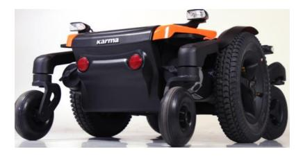
Each of the middle wheels is propelled by a powerful drive motor. These motors also take care for the steering of the wheelchair. With this system it is possible to turn on the spot. This makes the wheelchair optimal for indoor use.
