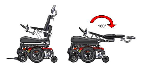
At a reclined backrest position over 135° the driving speed will be automatically reduced for safety reasons.
