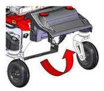
step 5. Unfasten the cable ties of the power module cables and pull it up to remove the plastic cover.
