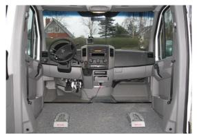
Dahl docking station mounted on the floor
