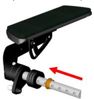
step 8: Put the axles back into the backrest frame and tighten the two central
