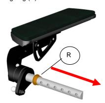
step 7: Add or remove the spacers of the axle and put the bearing back.
