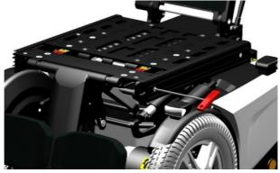
step 8: Mount the side rails into position and tighten the bolts.
