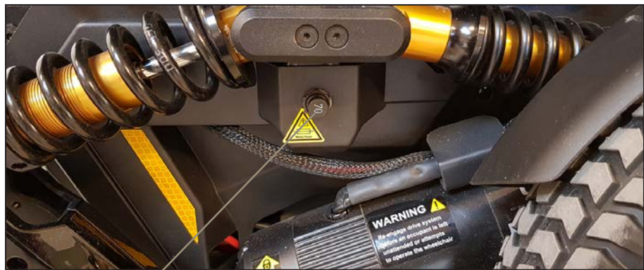
The automatic fuse is placed here.
