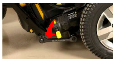
Position for disengagement - pushed down
