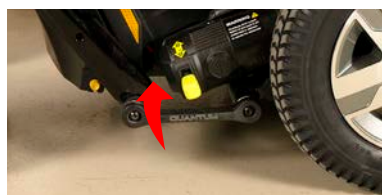
Normal position for driving - pushed up
