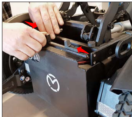
Push the lock pins toward the centre and flip the cover out.
