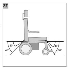
(see 9). Always take the total weight of the wheelchair into account in order to ensure that the tiedown system is the correct one.
