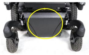
Position of the front maintenance free batteries
