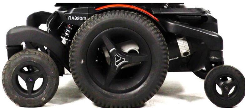
Each of the middle wheels is propelled by a powerful drive motor. These motors also take care for the steering of the wheelchair. With this system it is possible to turn on the spot. This makes the wheelchair optimal for indoor use.
