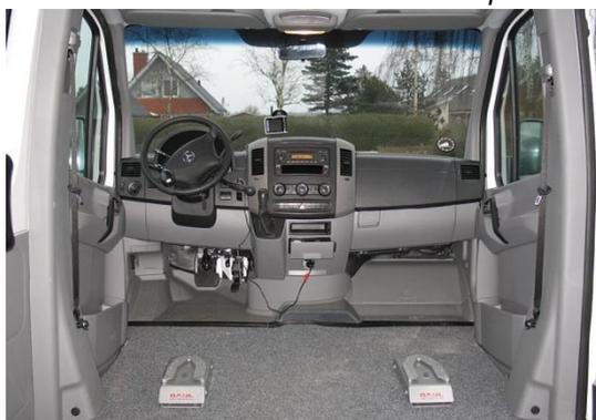
*Dahl Docking Station mounted on the floor*
