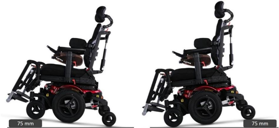
Driving down of a higher surface (like pavement), always be aware of the sudden forward movement of your wheelchair when driving down of it. If your wheelchair has powered seat tilt, you can use the seat tilt for more stability whilst driving of the pavement.
