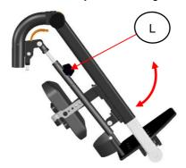
Step 1: To adjust and set the legrest angle, you hold the legrest with one hand and unlock the setting lever (L) with the other hand and push the legrest sideways.
