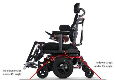
The straps have to be connected to the vehicle at suitable anchor points. Make sure that the tire pressure is at the recommended level so the straps
