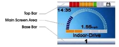
The color LCD screen is split into 3 areas of information. The Top Bar, the Base Bar and the Main Screen Area.
