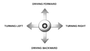
The secondary purpose of the joystick is to navigate through men menu of the wheelchair. By moving the joystick forward or backward you can scroll up or down through the menu, by moving to the right you can enter a sub selection.
