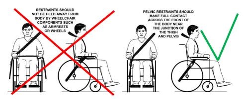
Picture of improper belt fit
