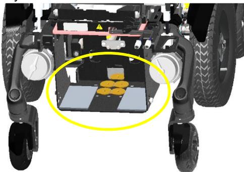
2. Place two plastic spacers (Dahl part no. 501910) in the battery box just like the drawing in the above. The best is to fix them with some double sided tape.
