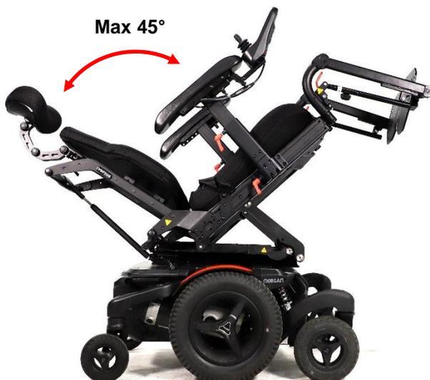
If the tilt is activated over a certain angle, the driving speed will be reduced. This is to reduce the risk of danger whilst driving at high speed.
