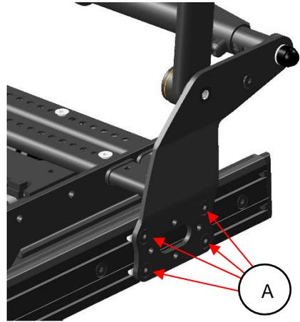
Step 1: Loosen the 4 bolts on each side of the backrest bracket (A) by using a 4mm Allen key.
