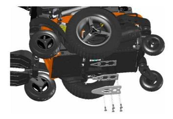
Mounting the Dahl docking plate on to the Morgan M Versus (MGNM-VRS) chassis
