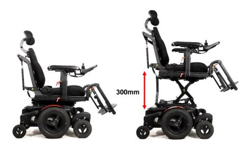
Whilst lifting the seat, the driving speed will always automatically be reduced to gain maximum stability. At high seating position also, the seat tilt will be blocked to gain maximum stability. The seat height can be set to every height position by the user.
