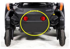
Position of the rear maintenance free batteries
