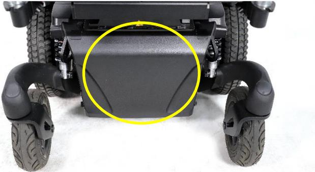
*Position of the front maintenance free batteries*
