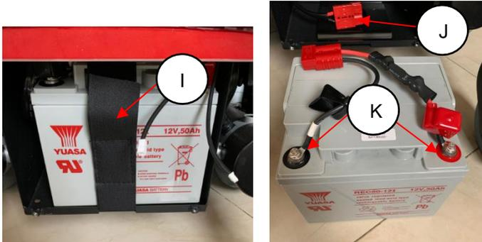
Step 5: take the new battery and then connect the cables on to the positive and negative poles.
