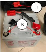
Step 5: take the new battery and then connect the cables on to the positive and negative poles.
