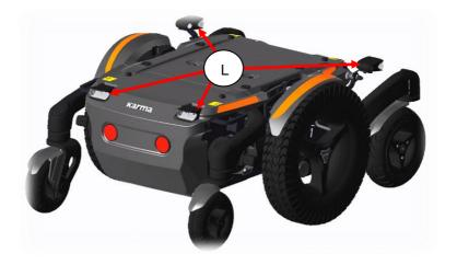
The chassis has very strong and bright LED lights to make sure you can have a safe drive in the dark. The red reflectors in the rear also make you visible for other people as well. The lights fulfill the European requirements. The additional LED indicators give our environment clear information in which direction you want to go.
