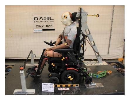
Morgan M Versus (MGNM-VRS) crash test using Dahl Docking Station
