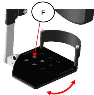
Step 2: Move the footplate to the required angle.
