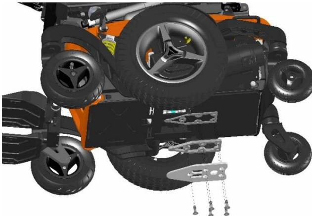
*Mounting the Dahl docking plate on to the Morgan M Versus (MGNM-VRS) chassis*
