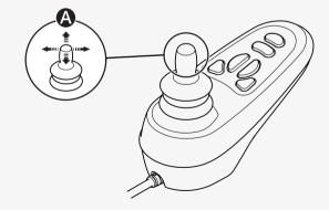
Do not move the joystick before, during, or immediately after you turn on the control system. If you move the joystick during this time, it can generate a joystick error. If this happens, turn the wheelchair off and then on.
