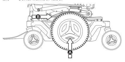
The serial number label is located on the lower, left-hand side of the wheelchair chassis. An additional serial number label is located on the seat tilt 3. You may need to tilt the seat to see the serial number label.
