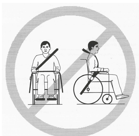
Illustration of improper belt-restraint fit
