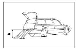
The load capacity of the ramp or lifting platform must be higher than the overall permitted weight of the electric wheelchair.
