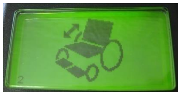
Picture B, joystick pressed to the left or right -> Tilt in space
