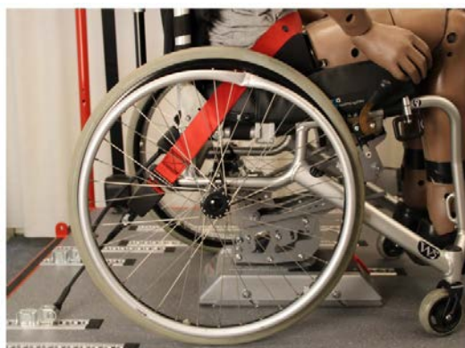
Occupant belt restraints must not be held away from the body by wheelchair components such as armrests or wheels
