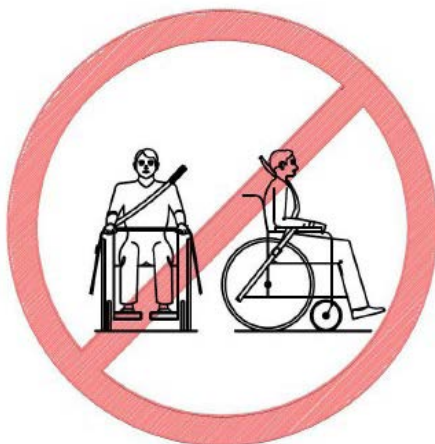
Illustration of improper belt restraint fit
