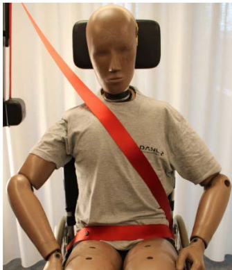
Occupant belt restraints must not be held away from the body by wheelchair components such as armrests or wheels
