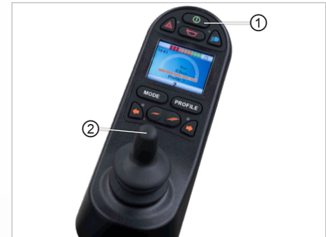
Fig. 88: Blocking the controls
