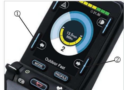
Fig. 52: Turn signal right / left
