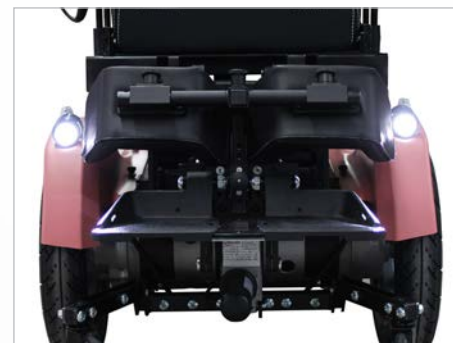
Fig. 97: Illumination at the front
