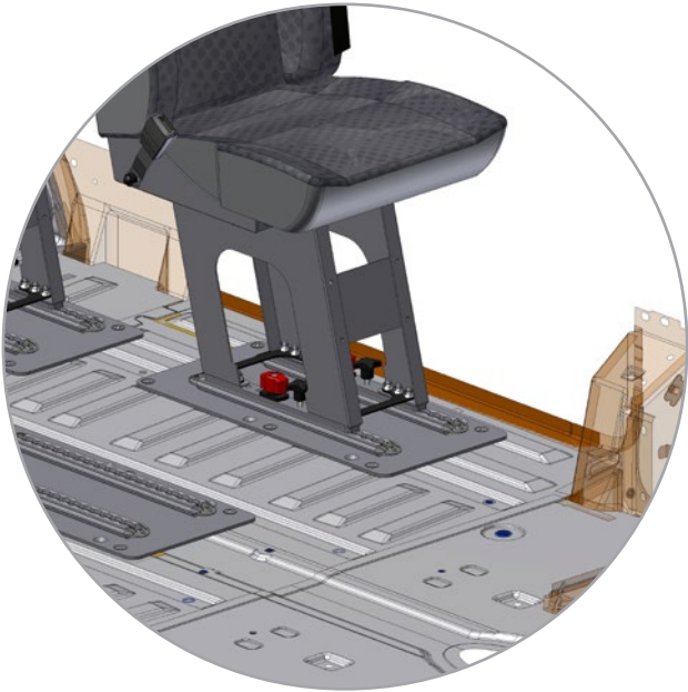
The reinforcement components are adapted to the installation point in question – including installation carried out around the fuel tank.
