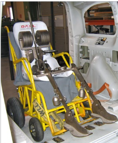
ECE regulation 17 H-point measurement
