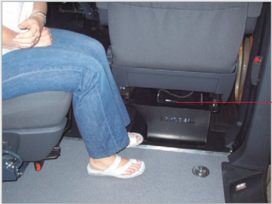
Seat base for original passenger seat, which provides approx. 10 cm more room for the feet when turning away from the driver's seat with a swivel seat base fitted.
