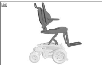
The power wheelchair is equipped with a combination of power seat tilt and seat height adjustment.
