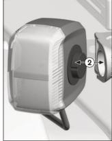
The front lighting consists of two LED headlights with integrated LED direction indicators (see fig. 37, item 1). The rear lighting consists of two LED rear lights with integrated direction indicators.
