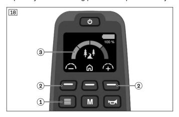
The limitation of the driving speed can be adjusted on the hand module using the [Softkey 1 - 3] buttons (see fig. 18):
