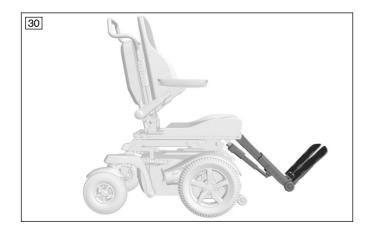
The centrally fitted leg support prevents a constant pressure load or provides anti-shock support.
