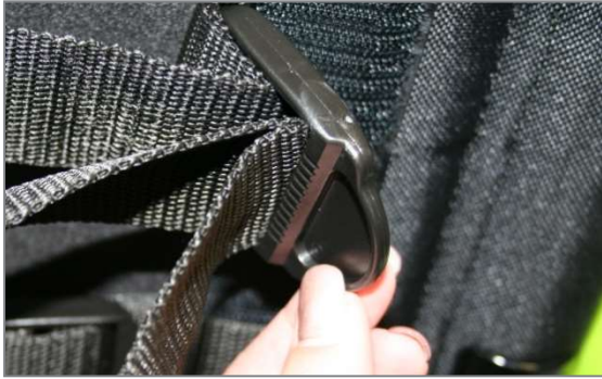
Figure 39: Step 5: Returning the belt through the tensioning loop to obtain the required "double passage"
