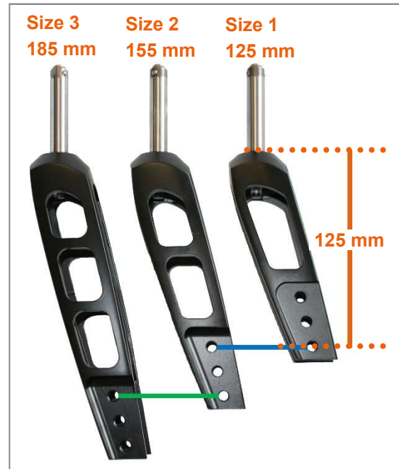
Figure 13: Caster fork sizes with marking of the same seat height settings with different caster fork sizes
