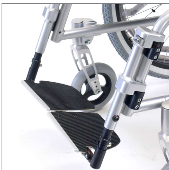
Figure 124: Swing away footrest, in standard position
