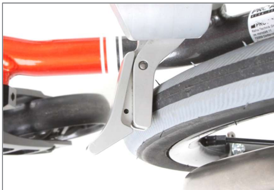
Figure 160: Brake element resting on the tyre
