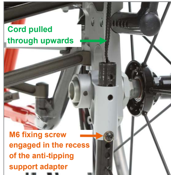
Figure 136: Anti-tipping bar inserted into the anti-tipping support adapter
