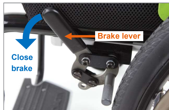
Figure 144: Brake opened; to close, push the brake lever forwards and downwards
