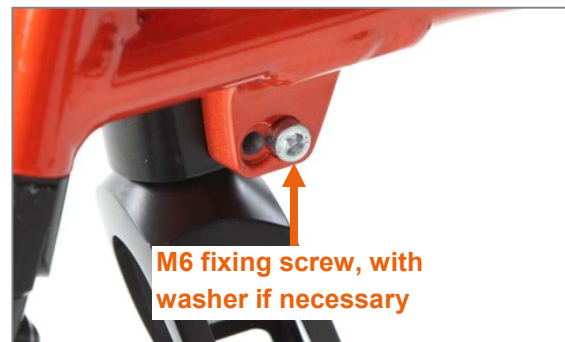
Figure 101: M6 fixing screw on frame inner side, washer fitted with G-shape frames but not V-shape frames
