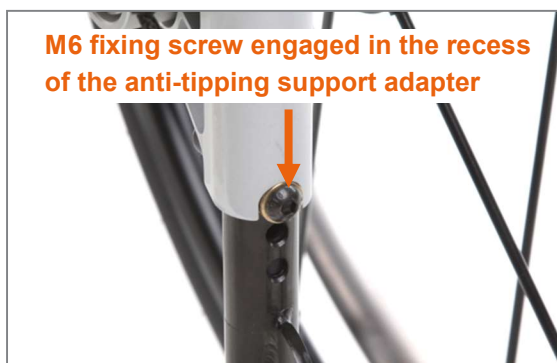
Figure 133: Anti-tipping support engaged correctly
