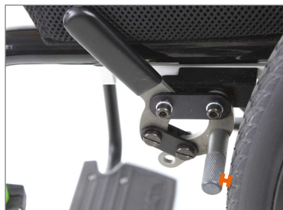
Figure 147: Distance between brake pin and tyre of approx. 3 mm to maximum 4 mm, with opened brake
