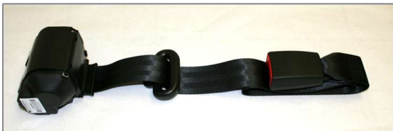
Figure 173: Automatic diagonal shoulder belt with deflector and buckle
