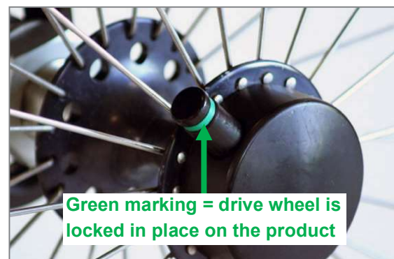
Figure 70: Tetra Clip with locked quick release axle
