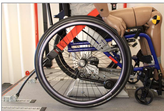
Figure 196: Occupant belt restraints must not be held away from the body by wheelchair components such as armrests or wheels
