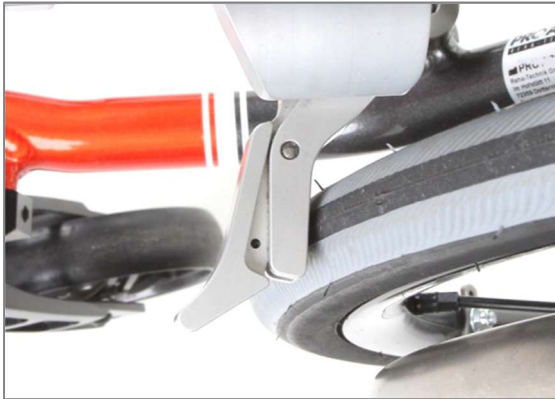
Figure 156: Brake element resting on the tyre
