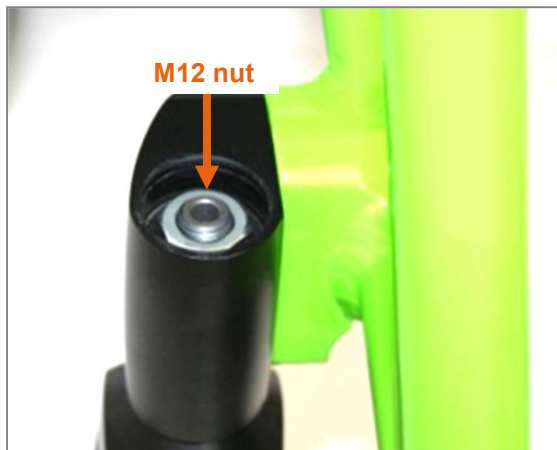
Figure 97: Aluminium cap removed and M12 nut visible
