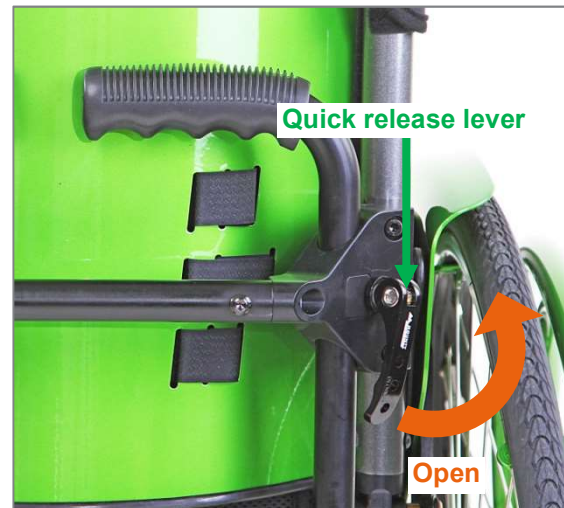
Figure 168: Closed quick release lever
