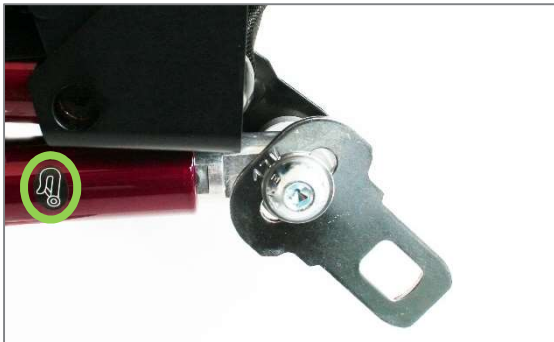
Figure 177: Transport restraint system attachment on the rear frame with latch plates for rear retractor and lap belt (view from the side)
