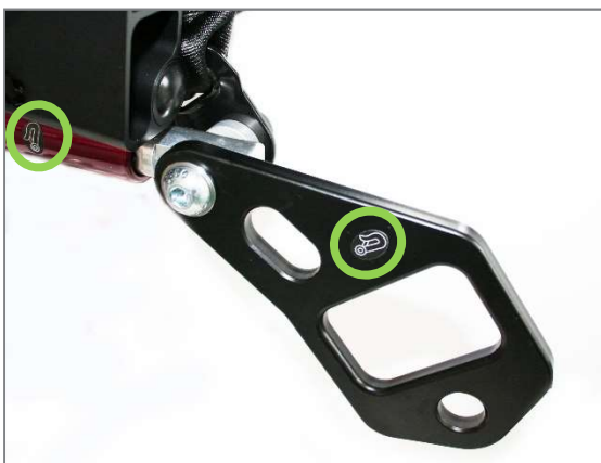
Figure 178: Transport restraint system attachment on the rear frame with belt eye for rear retractor and lap belt
