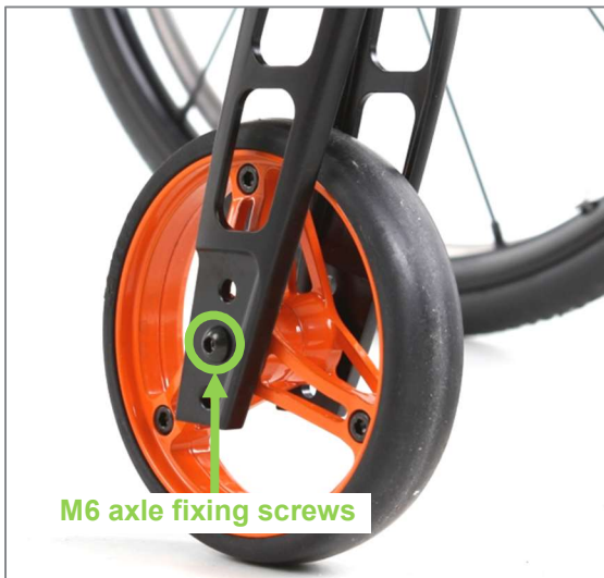
Figure 87: M6 axle fixing screw of caster wheel axle (view from outer side of product)
