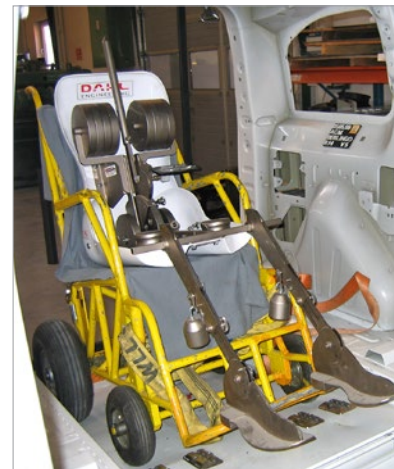
ECE regulation 17 H-point measurement
